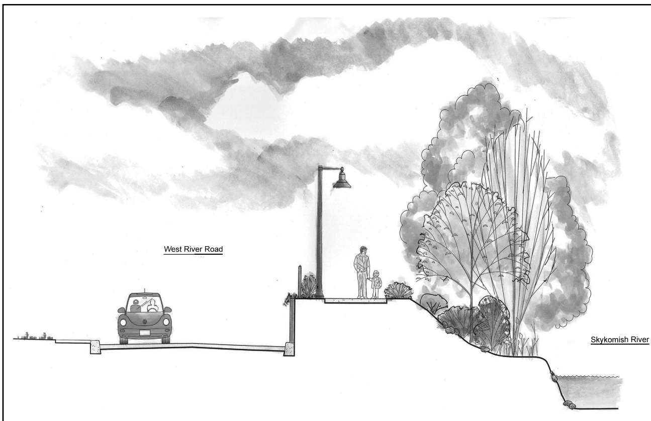
Cross section of proposed levee design
